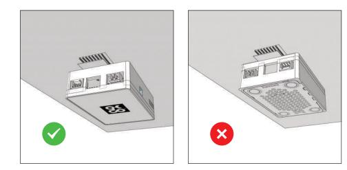
Place the Hubble control unit under your furniture or POS, as indicated above. Use the adhesive velcro band provided to fix the Hubble control unit.
