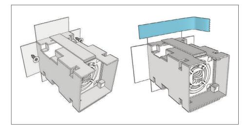
Fix the fan and the capsule inside your furniture or POS. The fan and capsule holder can be fixed with screws or scotch tap to your support, or by any efficient solution.
