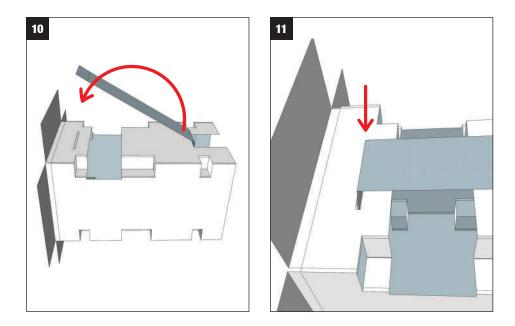
**10 I 11.** Insert the last strip band into the opening in order to secure a Scentys capsule. The support for the fan and capsule is now complete.
