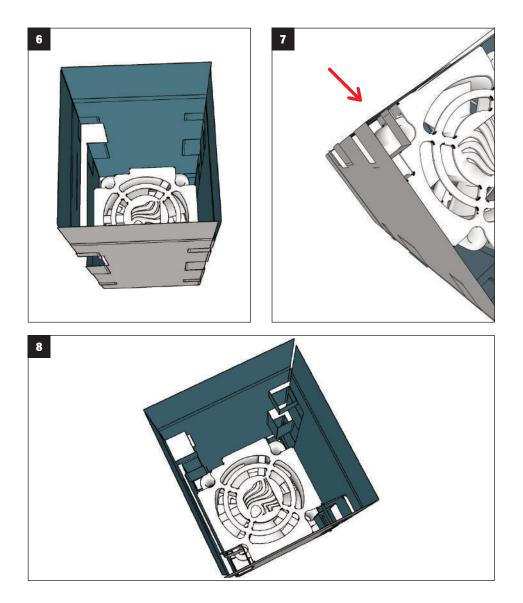
**6 I 7 I 8.** Push all the angles inside the holder to secure the fan position.
