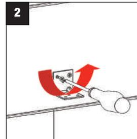
Screw the screws (not provided) into the wall (using dowels if necessary).
