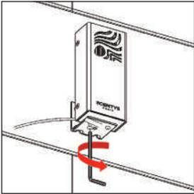
Attach the Scentys Pocket Duo using the screws provided and the Allen wrench.
