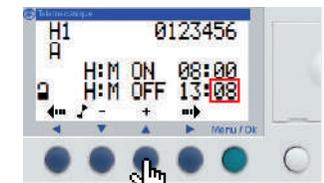
Press **▶** to access the stop minutes time value and change it if necessary by pressing **▲**. Clock parameter setting is complete, you can then go on to configure the intensity. 21/28
