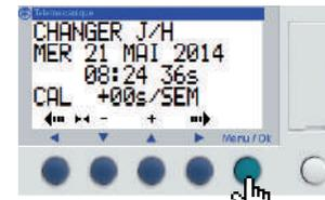
Once the parameters are correct, to return to the main menu, press **●** to exit the parameter setting pages.
