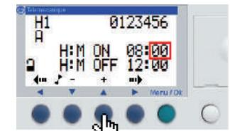
Press **▶** to access the start minutes time value and change it if necessary by pressing **▲**.
