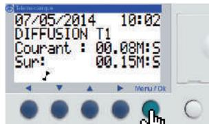
Press **Menu/OK** in normal operation to access the parameter setting menu.
