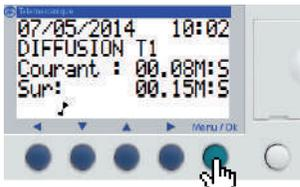
Press **●** in normal operation to access the parameter setting menu.
