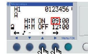
Press **▶** until the start time field is selected. Press **▲** to change the start hour time value.
